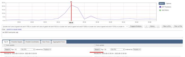
4. The Top-N tab is one of the most useful tools within NeMo analysis and contains information such as source IP, destination IP, percentage of traffic by any given IP, and packet rate. Once the Search button has been clicked, all this information will populate in the page. This process can be repeated for all other pages.
